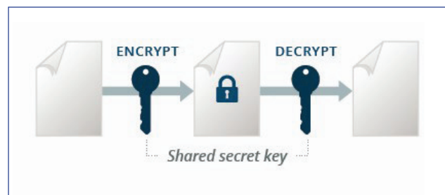
FIGURE 5: SYMMETRIC KEY ENCRYPTION
